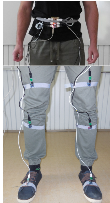
Fig. 4: Location of IMUs and control unit for gait sensing.
